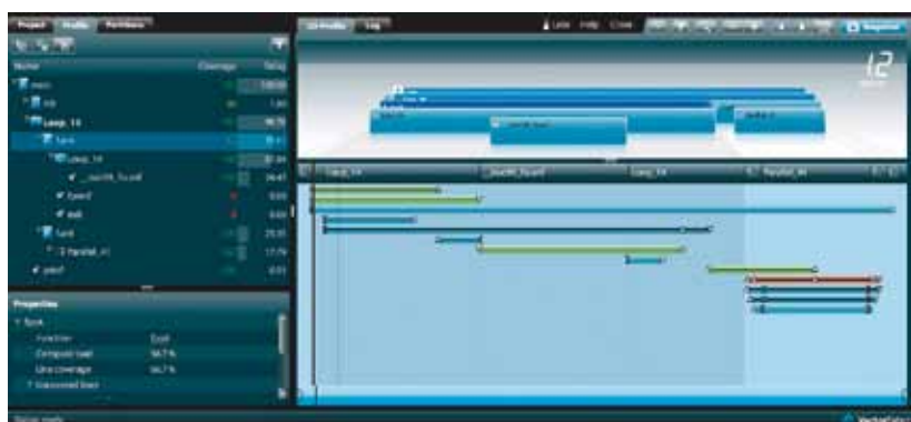
3D View of the program structure (upper part) and data dependencies (bottom): red dependencies create a serious challenge for partitioning; green ones can be managed by adding streaming channels after partitioning
